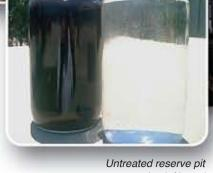
water (on left), and reclaimed water using the Green Machine
